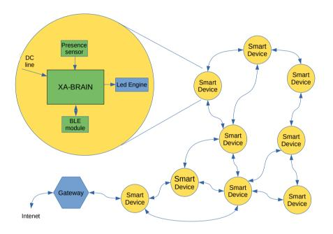
Figure 2: Block diagram of a connected system. The upper left yellow circle shows inner details of each smart device node
