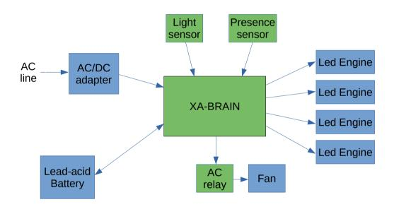
Figure 1: Block diagram of a standalone system
